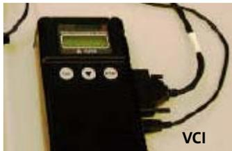
To install the Vehicle Communication Interface (VCI):
