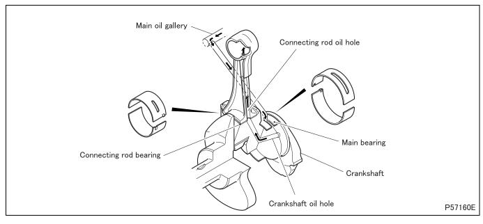
• Engine oil supplied through an oil passage in the crankshaft lubricates the big end (connecting rod bearing) of each connecting rod. Simultaneously, engine oil supplied through an oil passage in the connecting rod lubricates the connecting rod's small end.
