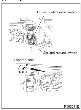
The operation of the auto cruise function using the set and resume switch is as follows:
