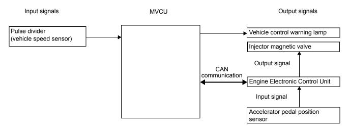
• The vehicle speed limiting (SLD) function is designed to send output signals to the engine ECU to restrict the maximum vehicle speed to a preset speed limit regardless of the accelerator pedal operation when the vehicle speed reaches the speed limit on flat or uphill road.
