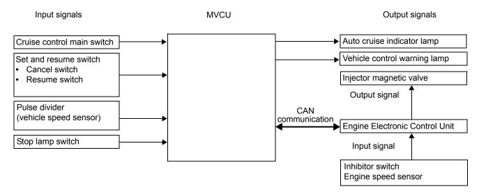
• In the auto cruise function, the target vehicle speed is set using the main switch, set switch and resume switch, and the MVCU maintains the set speed by controlling the engine.
