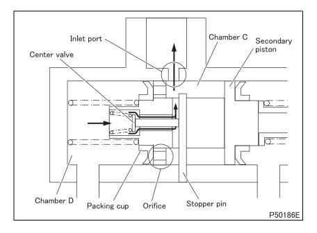
With the secondary piston back in its original position, there is no difference in fluid pressure between chambers C and D. The packing cup restores its original shape, blocking the orifices. The liquid pressure in the brake line now flows through the center valve, which has been open since hitting the stopper pin. The liquid pressure then returns through the inlet port to the brake fluid tank.
