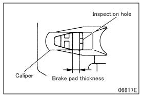
• Through the inspection hole in the caliper, measure the brake pad thickness. If the measured value is less than the limit, replace all of the brake pads on that axle with a new kit.
