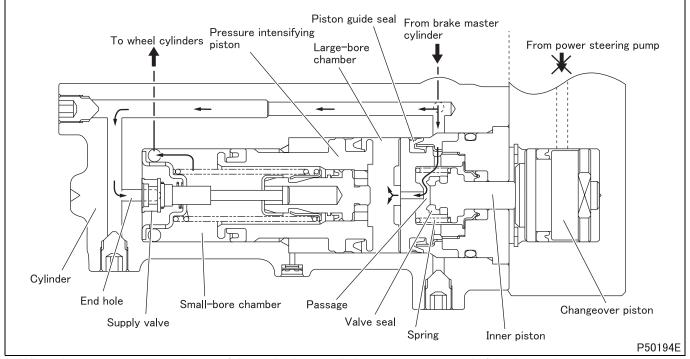
When the power steering oil pump fails to discharge oil, the spring at the end of the inner piston pushes back the inner and changeover pistons. This opens up the passage through the valve seal into the large-bore chamber.
