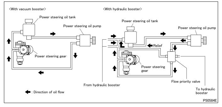
• The power steering system with hydraulic booster is provided with a flow priority valve to reduce steering shock that occurs when the brakes are suddenly applied during steering wheel manipulation.
