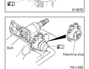
• Tighten bolt to the specified torque, then retighten the adjusting plug using *[*, ].
