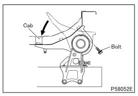
• Lower the cab all the way, then remove bolt.
