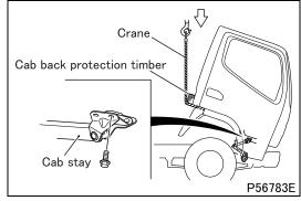
• Supporting the tilted cab with the crane, remove the cab stay.
