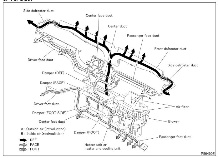
• The blower sends outside air **A** or inside air **B** through the heater unit or heater and cooling unit to the ducts. The flow of air is dependent on the open/closed positions of the various dampers.
