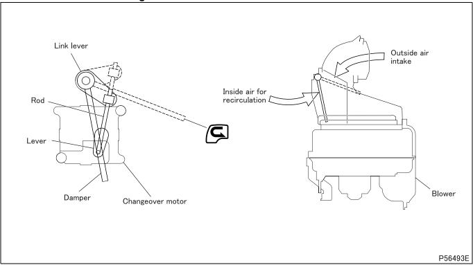
• The fresh/recirculation changeover damper is operated by means of motor.
