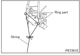
In order that the control cables can be pulled back at the time of installation, attach string to the ring parts of the cables as shown in the illustration.
