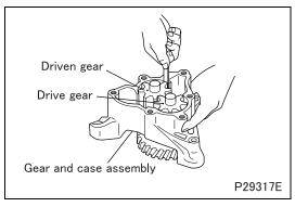
(2) Gear and case assembly-to-tooth tip clearance for each gear
