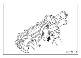
• Remove the engine oil pressure switch.
