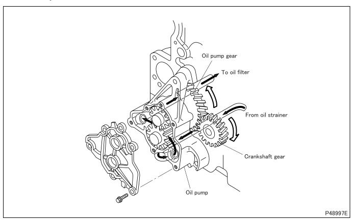
• This engine uses a gear-type oil pump driven by the rotation of the crankshaft transmitted through the engagement of the crankshaft gear and the oil pump gear.
