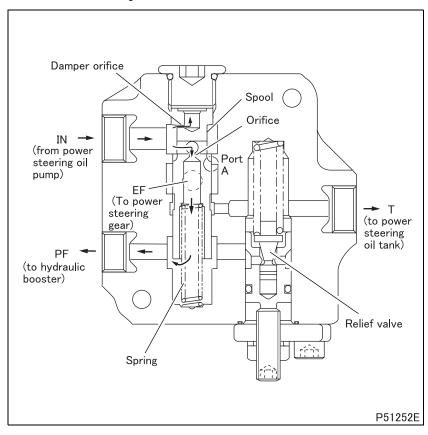
When brakes are applied hard while the steering wheel is turned, the flow priority valve dampens the associated steering shock by appropriately distributing the flow from the power steering oil pump between the hydraulic booster and the power steering gear.
