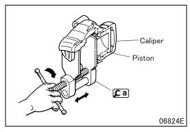
• Using the piston expander **[a]**, screw in the piston of the caliper until it bottoms on the back of the caliper.
