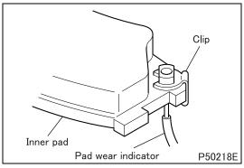
Install a pad wear indicator onto the inner pad (included in the pad kit) using a clip (included in the pad wear indicator kit).
