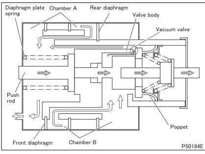
In further progression, the poppet separates from the valve body. This opens the vacuum valve, allowing vacuum from the vacuum pump to flow into chamber B. As there is now no pressure difference between chambers A and B, the diaphragm plate spring pushes back the front and rear diaphragms and also the push rod to their original positions.
