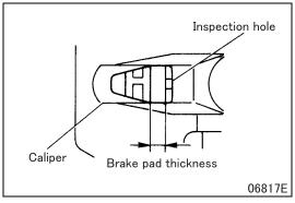
Through the inspection hole in the caliper, measure the brake pad thickness. If the measured value is less than the limit, replace all of the brake pads on that axle with a new kit.
