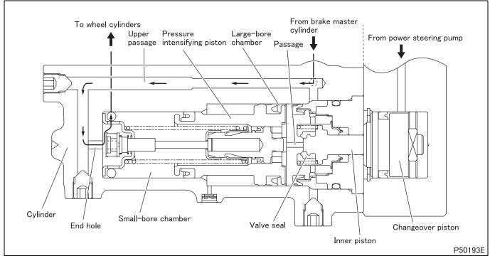
Power steering oil pump pressure pushes the changeover piston, which then moves the inner piston. As a result, the passage to the large-bore chamber is blocked by the valve seal. Fluid pressure from the brake master cylinder flows through the upper passage, the end hole, the small-bore chamber, and into the wheel cylinders. As fluid pressure acts only on the small-bore end of the pressure intensifying piston, the piston remains in the same position.
