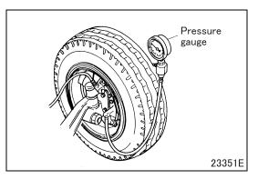
• If any fault is observed during these checks, replace the hydraulic booster.
