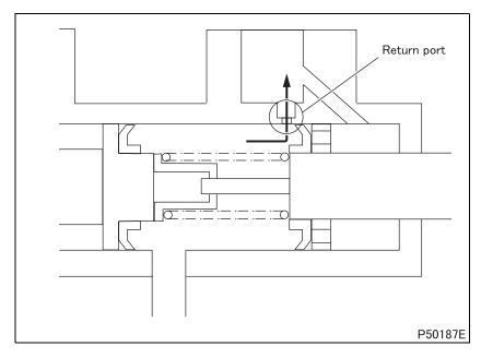
The fluid pressure in the primary (front) brake line returns through the return port to the brake fluid tank.
