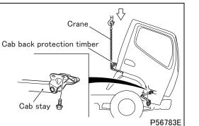
• Supporting the tilted cab with the crane, remove the cab stay.
