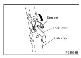
After the cab stay is installed, tilt the cab to securely lock the cab stay. Then, remove the crane from the cab.
