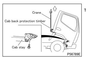
• Before tilting, support the cab using the crane. Tilt the cab with the crane, and install the cab stay.
